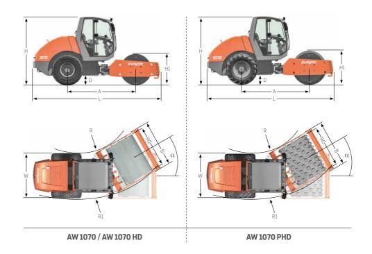
Distance between axles (A) 2,720 mm Width (B) 1,850 mm Road clearance (D) 375 mm Height (H) - AW 1070 (H) 2,723 mm - AW 1070 HD (H) 2,723 mm - AW 1070 PHD (H) 2,728 mm Drum diameter - AW 1070 (H1) 1,250 mm - AW 1070 HD (H1) 1,250 mm - AW 1070 PHD (H1) 1,140 mm Length (L) 5,032 mm Turning radius - inside (R) 3,900 mm - outside (R1) 5,600 mm 1,700 mm Drum width (W1) 1,700 mm Steering angle ( $\alpha$ )
