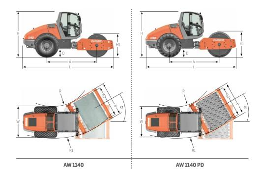
Distance between axles (A) 3,195 mm Width (B) 2,270 mm Road clearance (D) 490 mm Height (H) - AW 1140 (H) 2,920 mm - AW 1140 PD (H) 2,920 mm Drum diameter - AW 1140 (H1) 1,500 mm - AW 1140 PD (H1) 1,390 mm Length (L) 5,757 mm Turning radius 4,860 mm - inside (R) 7.015 mm - outside (R1) Width about tyres (W) 2,090 mm Drum width (W1) 2,100 mm Steering angle ( $\alpha$ )
