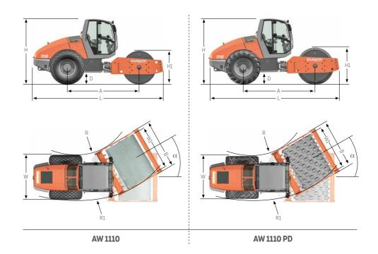
Distance between axles (A) 3,195 mm Width (B) 2,270 mm Road clearance (D) 490 mm Height (H) - AW 1110 (H) 2.920 mm - AW 1110 PD (H) 2.920 mm Drum diameter - AW 1110 (H1) 1,500 mm - AW 1110 PD (H1) 1,390 mm Length (L) 5,757 mm Turning radius 4,860 mm - inside (R) 7.015 mm - outside (R1) Width about tyres (W) 2,090 mm Drum width (W1) 2,100 mm Steering angle ( $\alpha$ )
