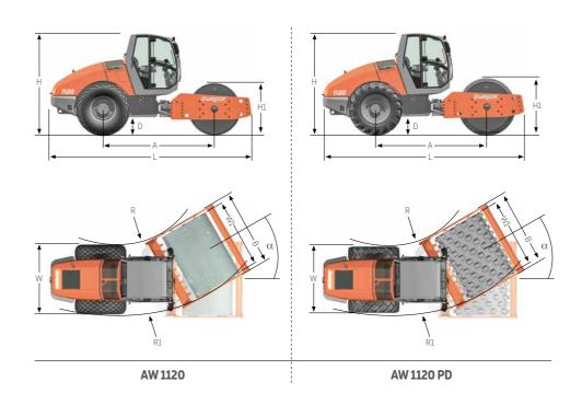
Distance between axles (A) 3,195 mm Width (B) 2,270 mm Road clearance (D) 490 mm Height (H) - AW 1120 (H) 2,920 mm - AW 1120 PD (H) 2,920 mm Drum diameter - AW 1120 (H1) 1,500 mm - AW 1120 PD (H1) 1,390 mm Length (L) 5,757 mm Turning radius 4,860 mm - inside (R) 7.015 mm - outside (R1) Width about tyres (W) 2,090 mm Drum width (W1) 2,100 mm Steering angle ( $\alpha$ )
