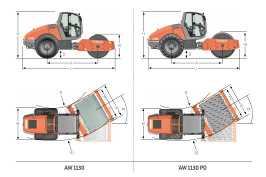
Distance between axles (A) 3,195 mm Width (B) 2,270 mm Road clearance (D) 490 mm Height (H) - AW 1130 (H) 2,920 mm - AW 1130 PD (H) 2,920 mm Drum diameter - AW 1130 (H1) 1,500 mm 1,390 mm - AW 1130 PD (H1) Length (L) 5,757 mm Turning radius 4,860 mm - inside (R) 7.015 mm - outside (R1) Width about tyres (W) 2,090 mm Drum width (W1) 2,100 mm Steering angle ( $\alpha$ )
